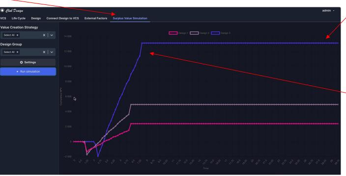
the simulation allows to confirm or disconfirm the initial rank-weight set in the value creation strategy (e.g. in the trade-off among thrust and lsp)
